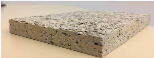
Front of rupture of a wood–cement particleboard cut with a saw
